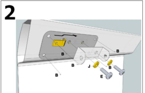
Offer the Holding Base Bracket through the 13mm hole to align with correspondingh holes in drilled Shelf Rail.
