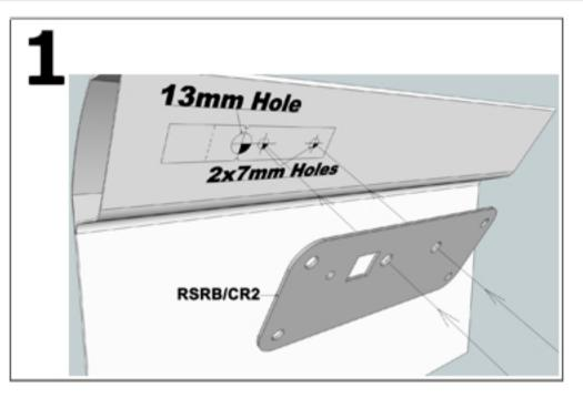
Use a centre punch on all drill centres. When drilling the holes ensure drills do not come in contact with outside skin.
